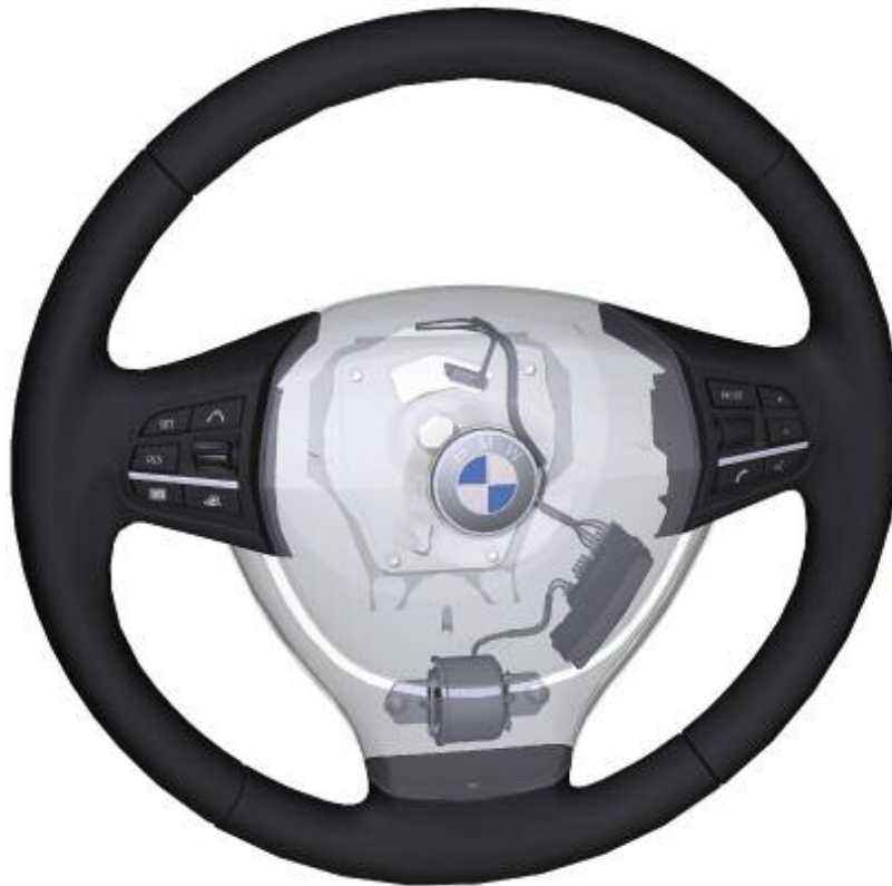
Lane departure warning vibration actuator
